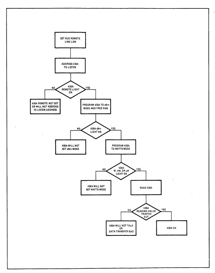
Figure 3-7. Test of HP-IB Operation Flowchart
