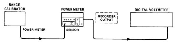
Figure 5-5. A-D Converter and Linear Meter Adjustment Setup
