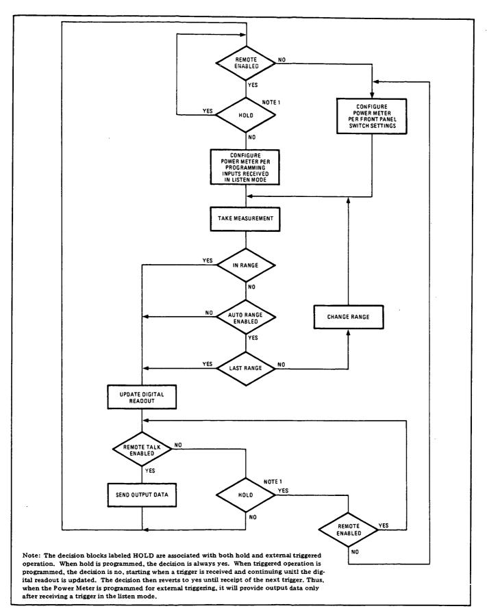
Figure 3-6. Operating Program Simplified Flow Chart
