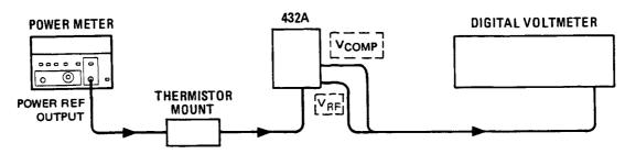
Figure 4-4. Power Reference Level Test Setup
