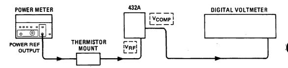
Figure 5-7. Power Reference Oscillator Level Adjustment Setup
