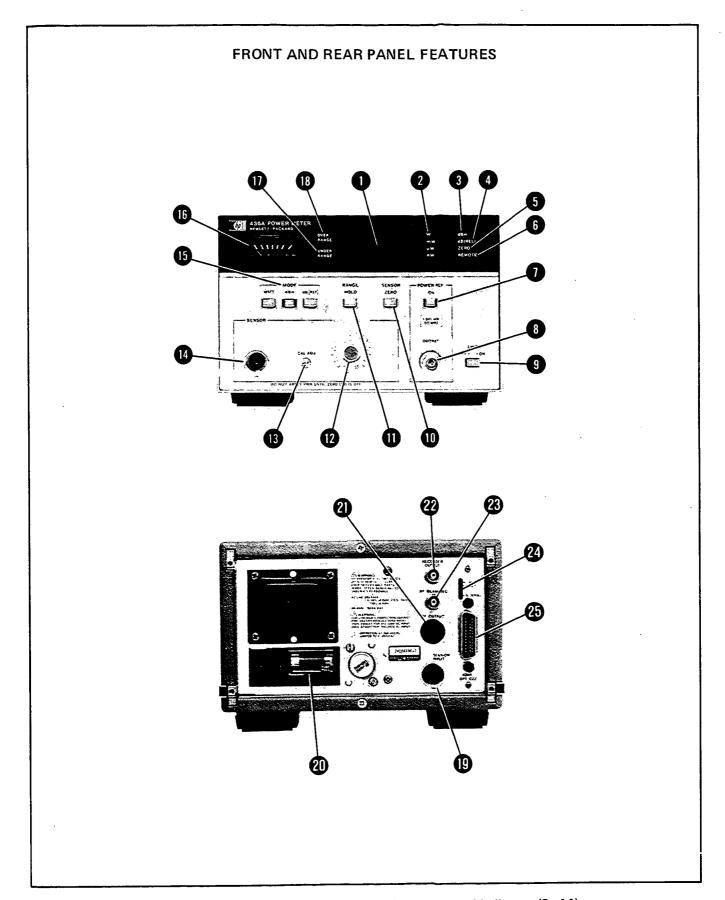
Figure 3-1. Front and Rear Panel Controls, Connectors, and Indicators (3 of 4)
