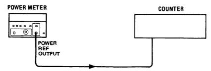
Figure 5-6. Power Reference Oscillator Frequency Adjustment Setup
