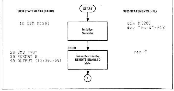
Figure 3-8. 436A Quick Programming Guide (1 of 5)
