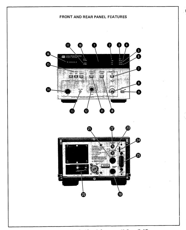
Figure 3-1. Front and Rear Panel Controls, Connectors, and Indicators (1 of 4)
