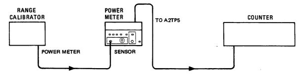
Figure 5-4. Multivibrator Adjustment Setup
