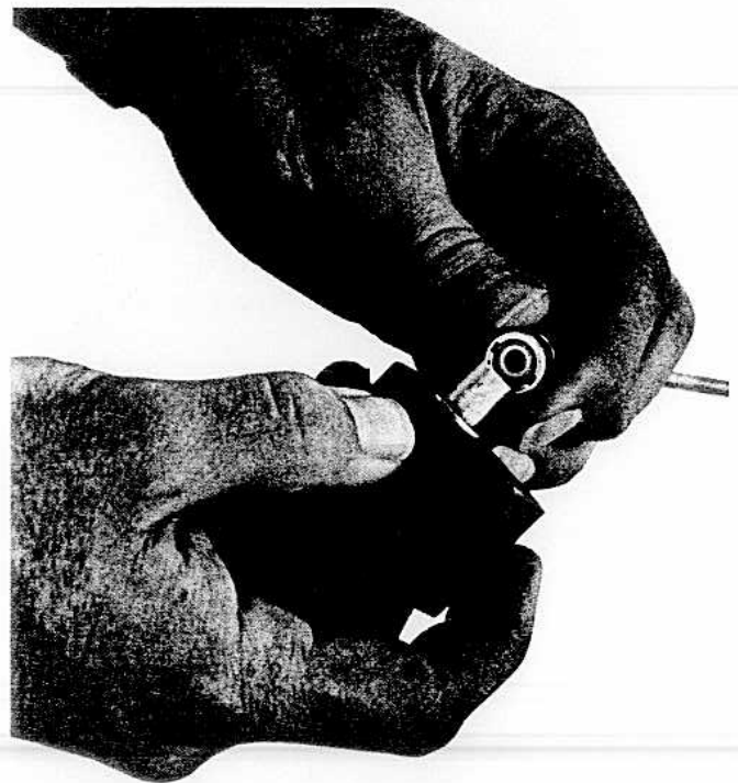
Figure 3. Discharging Cable before Connecting to Mixer
